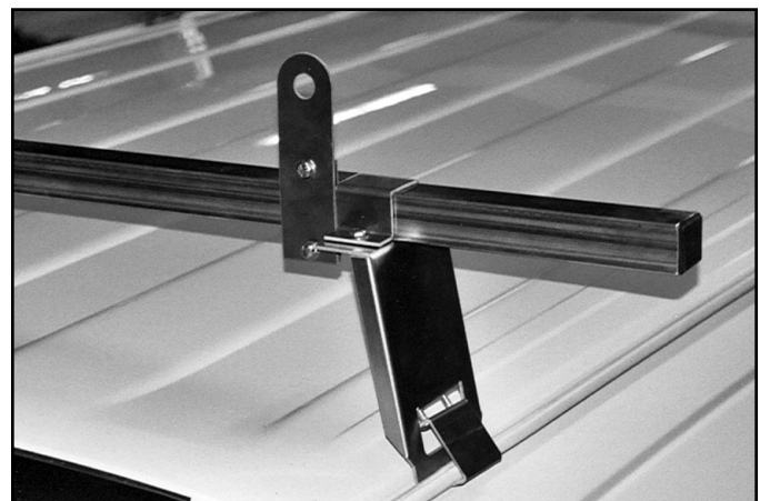
Photo of installed roof rack.
